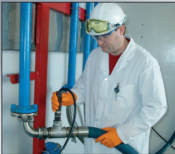
Rob Pastushak, senior technical/operational supervisor at Gil-ead Sciences' Alberta, Canada, facility inspects a pH sensor.
