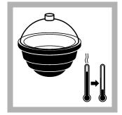
2. Remove the dish from the oven. Let the dish temperature decrease to room temperature in a desiccator.
