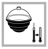
7. Remove the dish from the oven. Let the dish temperature decrease to room temperature in a desiccator.
