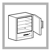
1. Put an aluminum dish in a drying oven at 103–105 °C (217–221 °C) for 1 hour.
