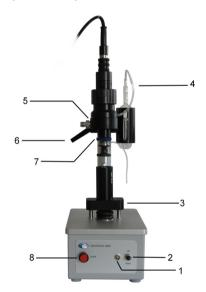
The PharmaPack can analyze volumes as small as one milliliter, in ampoules and vials. The oxygen sensor makes headspace gas measurements and sends them to the analyzer for display. The package sampler is operator controlled. Position of the sample platform controls the flow of purge gas.
