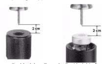
Loosen the black handle and adjust height of arm until the needle is 2 cm above the top of the ampoule package support (left photo) or the vial septum (right photo). Then, tighten the handle.
